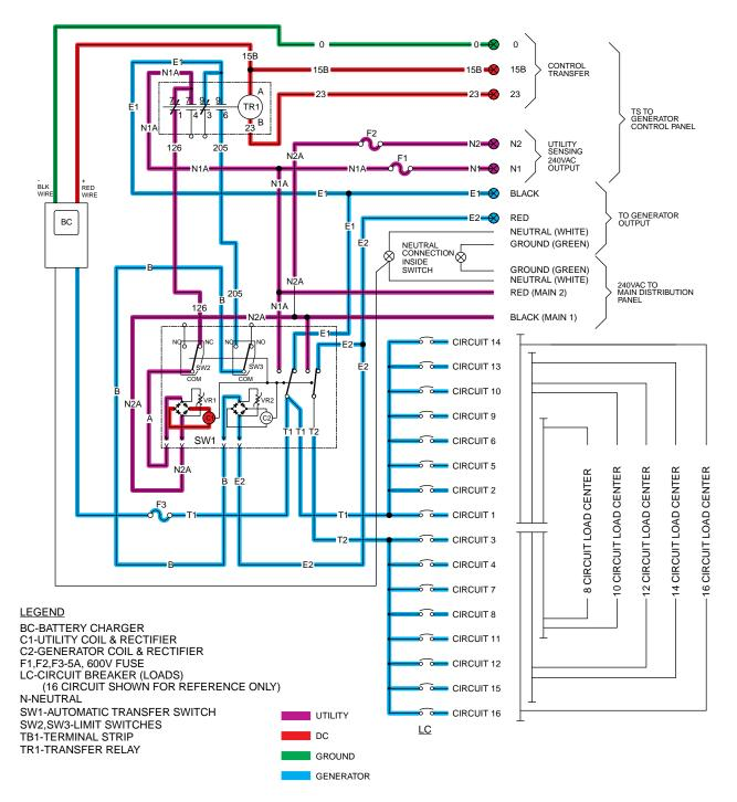
Figure 8. Utility Restored, Transfer Relay De-energized.
